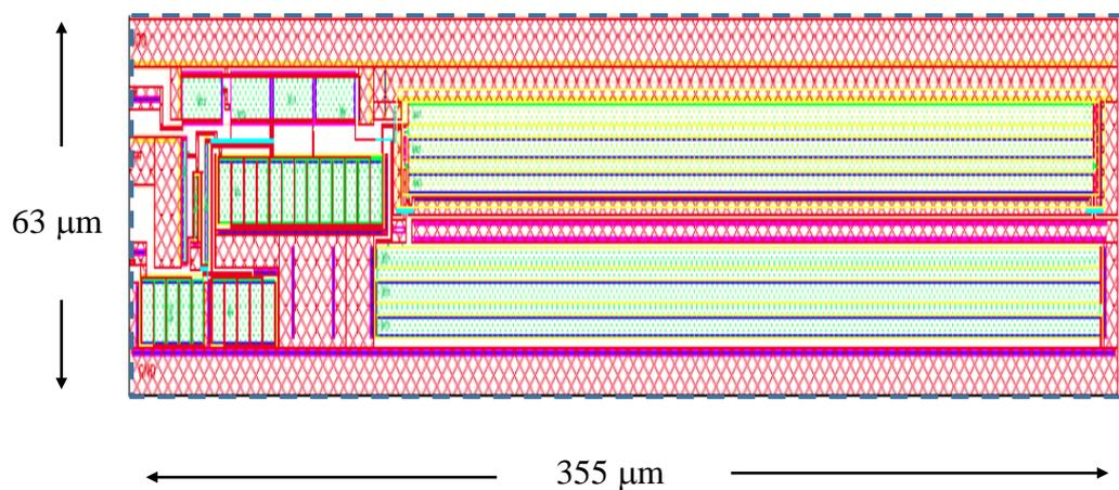
Fig. 4.6. Layout of the proposed current reference circuit.
