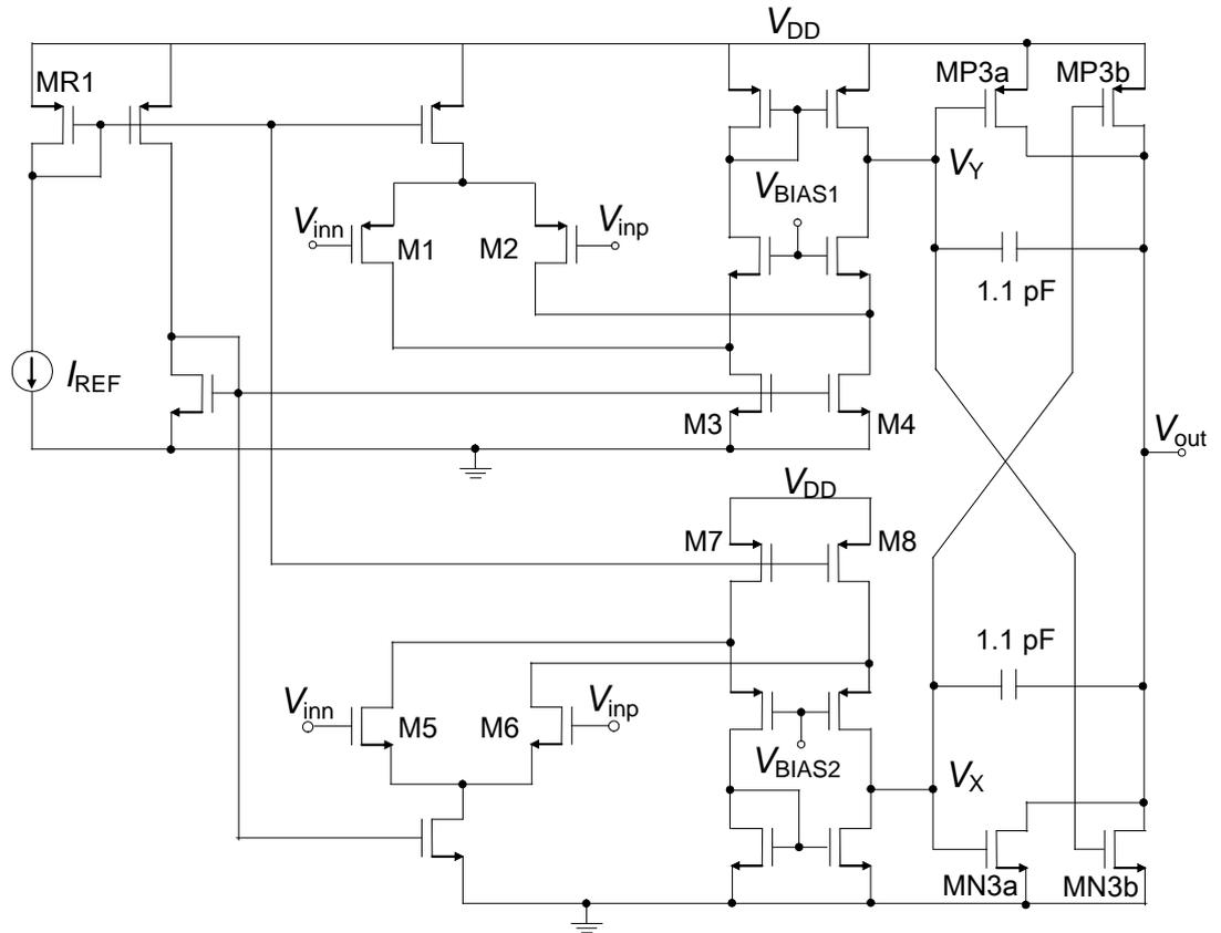
Fig. 3.2. Proposed rail-to-rail op-amp with a cross-coupled output stage.
