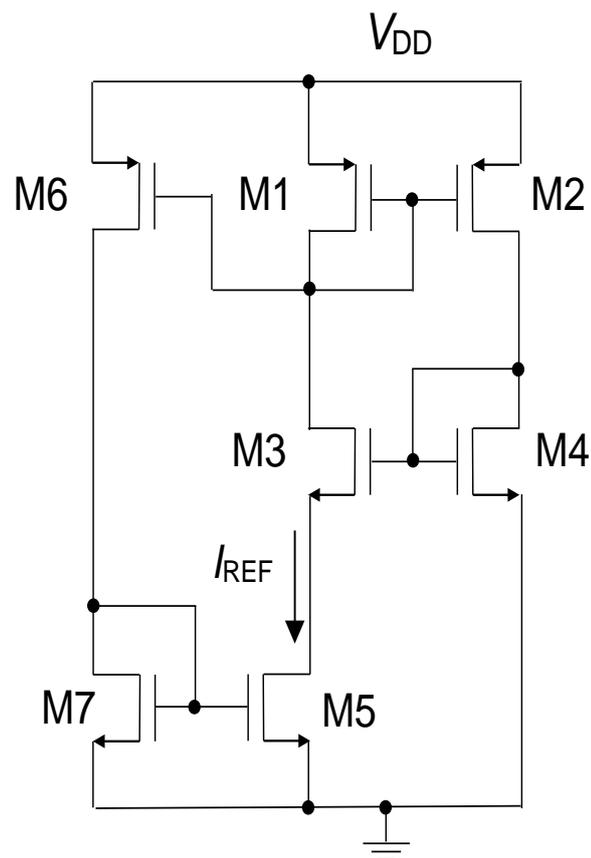
Fig. 4.2. Resistorless current reference circuit [10].
