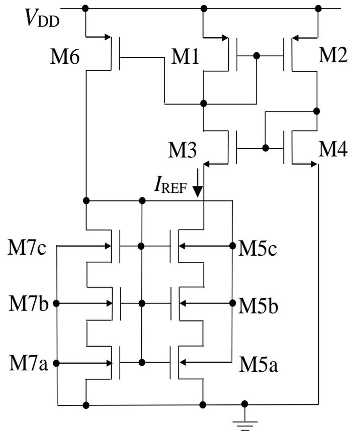
Fig. 4.5. Proposed current reference circuit using the self-cascode structure.
