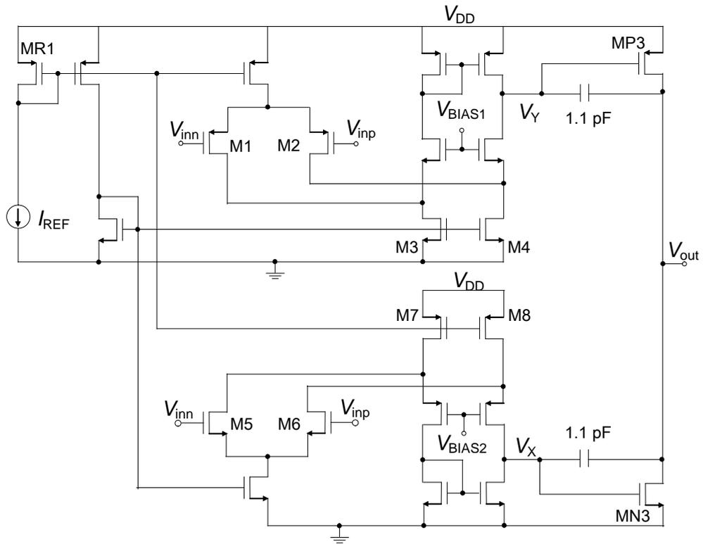
Fig. 3.12. Rail-to-rail op-amp with a common-source output stage.
