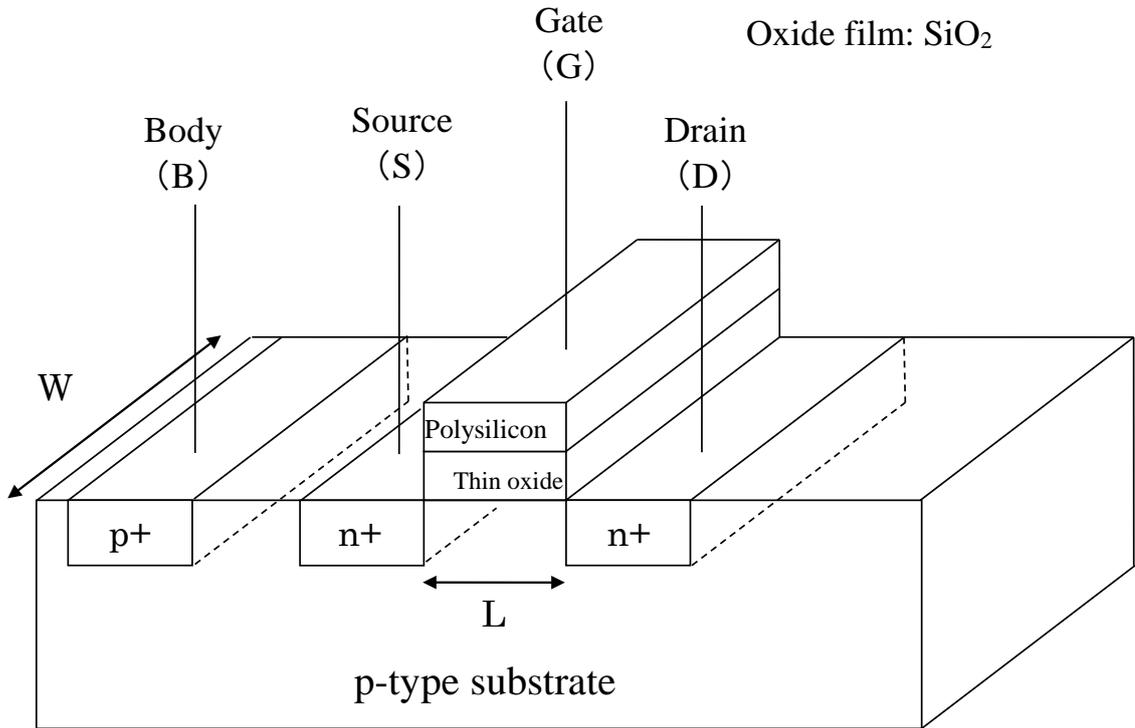
Fig. 2.1. Structure of a MOS device.
