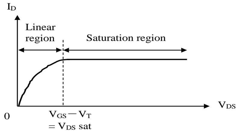
Fig. 2.3. Current-voltage characteristics ( $I_D - V_{DS}$ ) [2].
