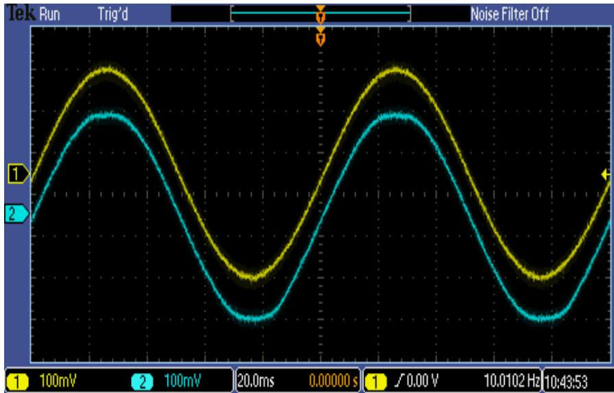
Fig. 3.17. Measured rail-to-rail input (yellow line) and output (blue line) waveforms with a 0.5-V supply voltage [18].
