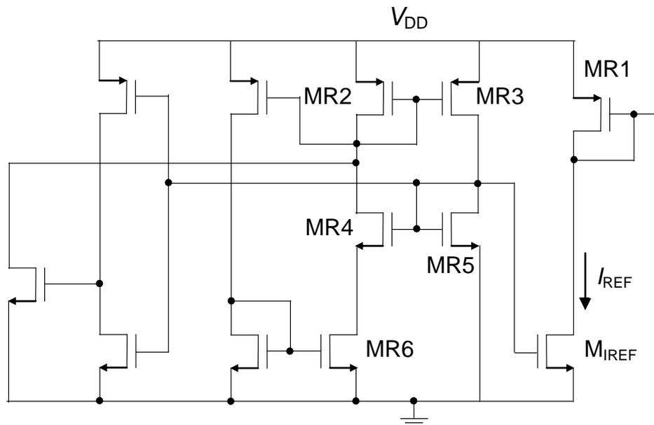
Fig. 3.4. Reference-current generation circuit [10].
