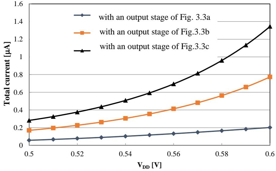
Fig. 3.8. Supply-voltage dependence of total current consumption.
