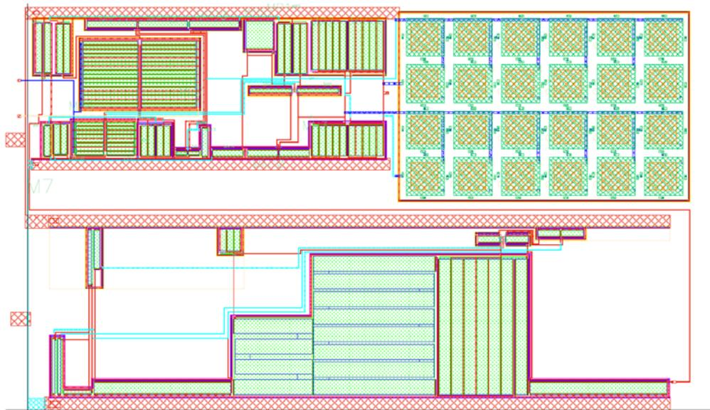
Fig. 3.15. Layout of the op-amp [18].
