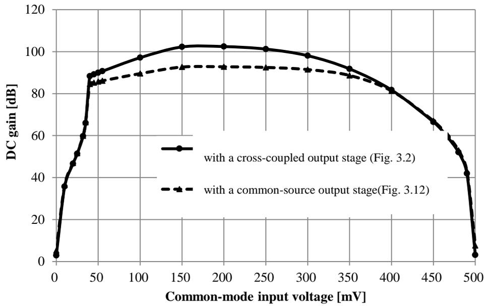
Fig. 3.9. DC gain and common-mode input voltage.
