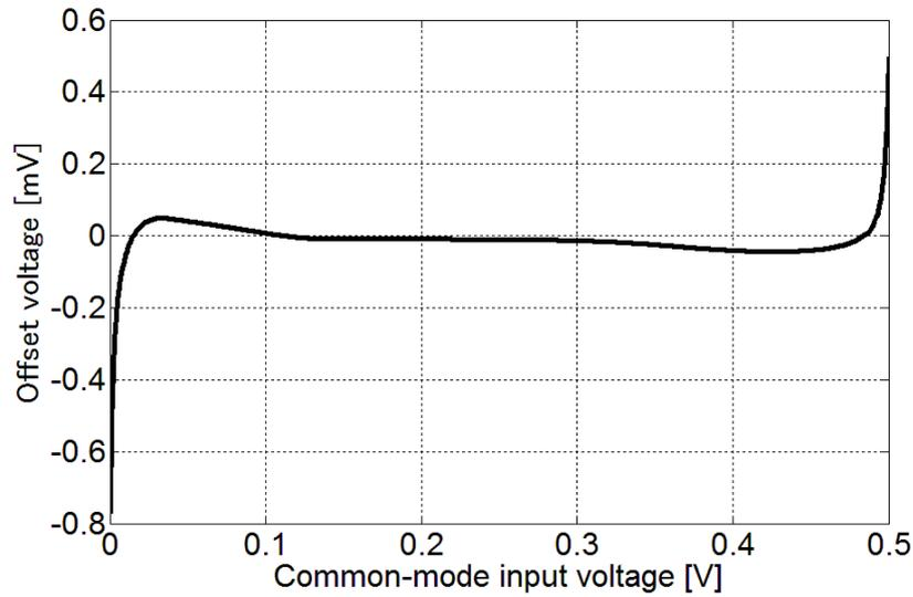
Fig. 3.6. Voltage difference between the input and output in a voltage-follower configuration.
