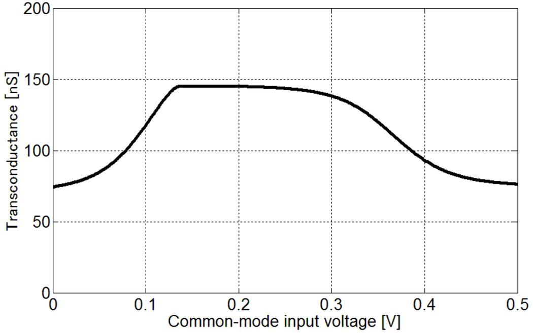
Fig. 3.10. Transconductance and the common-mode input voltage.
