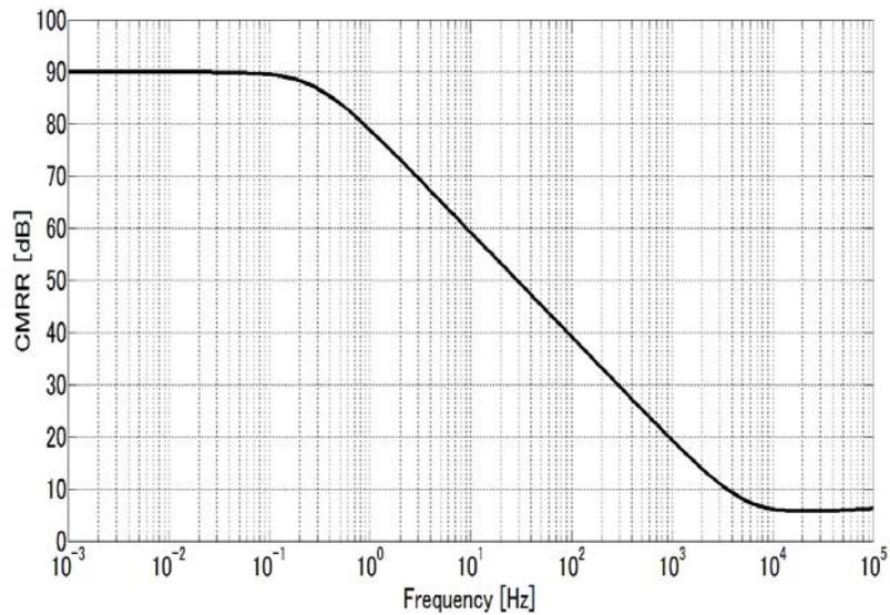
Fig. 3.11. Common-mode rejection ratio (CMRR).
