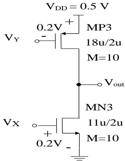
Fig. 3.3 (a). Conventional common-source output stage [18].
