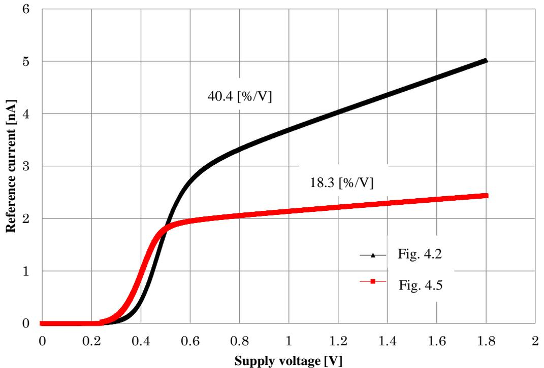
Fig. 4.7. The line regulation of conventional current reference circuit.
