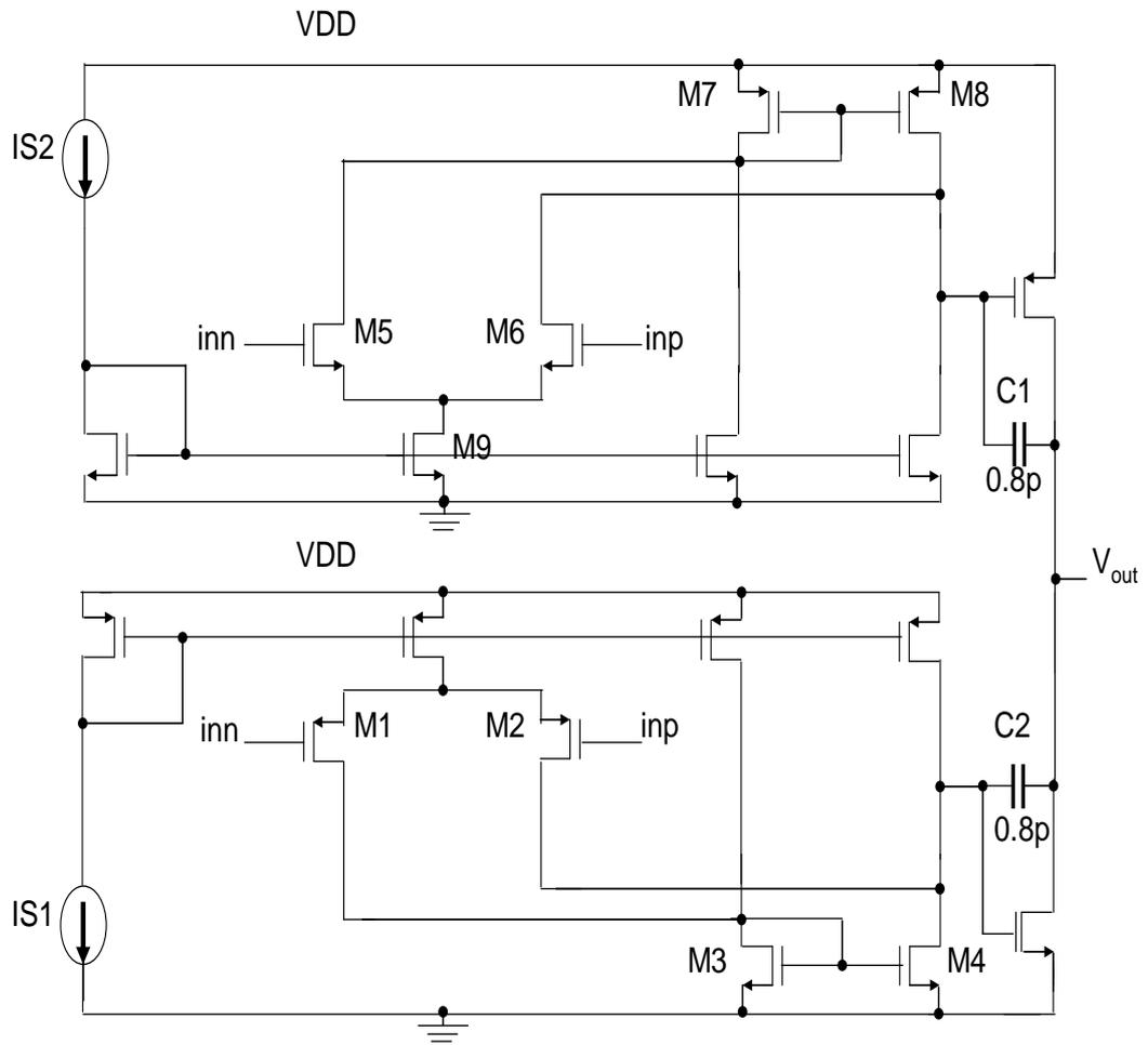
Fig. 3.1. Rail-to-Rail op-amp with a standard CMOS technology [9].
