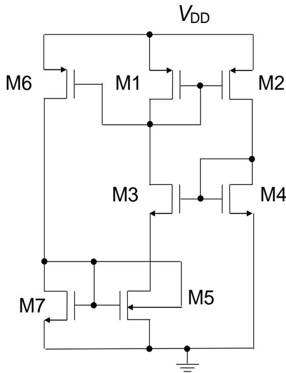
Fig. 4.4. Proposed CMOS current reference circuit
