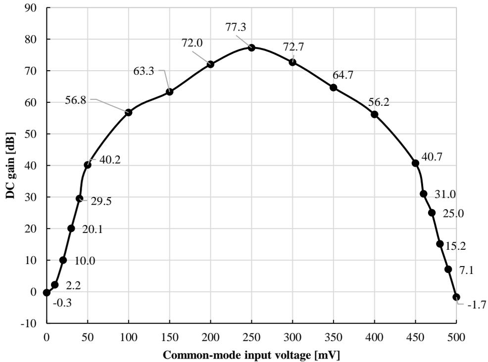
Fig. 3.19. Measured DC gain and common-mode input voltage [18].
