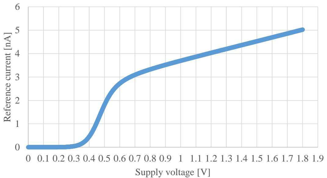
Fig. 3.13. Simulation result of the reference current circuit used in the op-amp.
