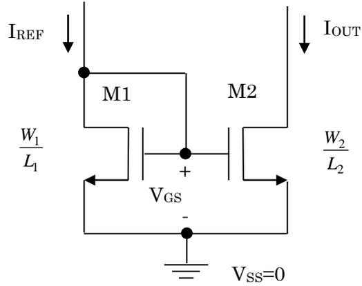
Fig. 2.4. A simple CMOS current mirror [1].
