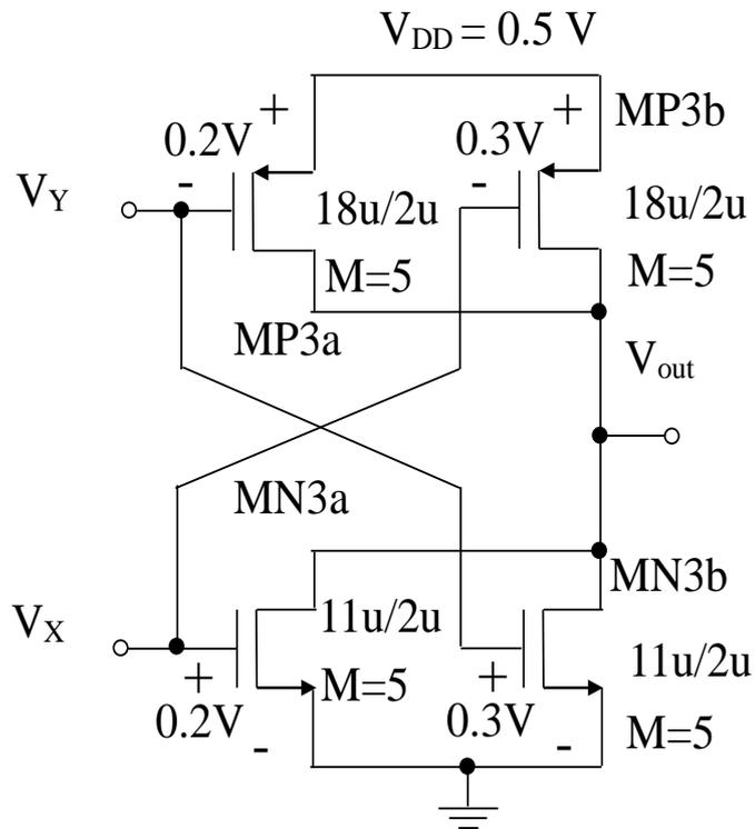
Fig. 3.3 (b). Proposed cross-coupled output stage.
