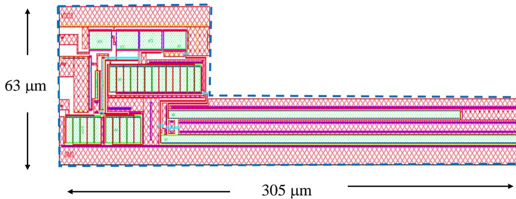
Fig. 4.3. Layout of the conventional current reference circuit (Fig. 4.2).
