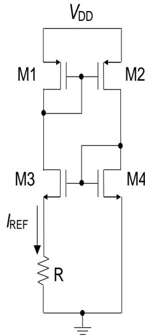
Fig. 4.1. Beta-multiplier current reference circuit [20].
