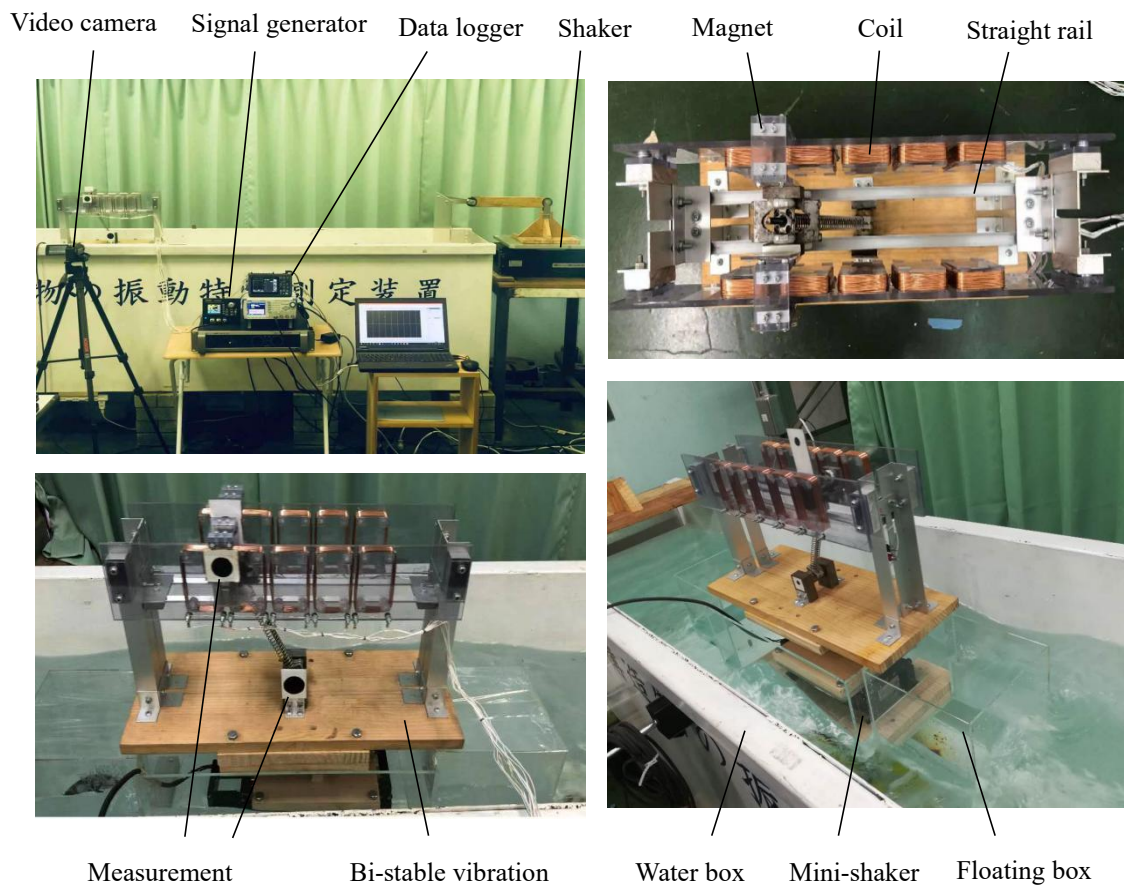
Fig.5-8 Photos of experimental settings of bi-stable vibration power generation system
