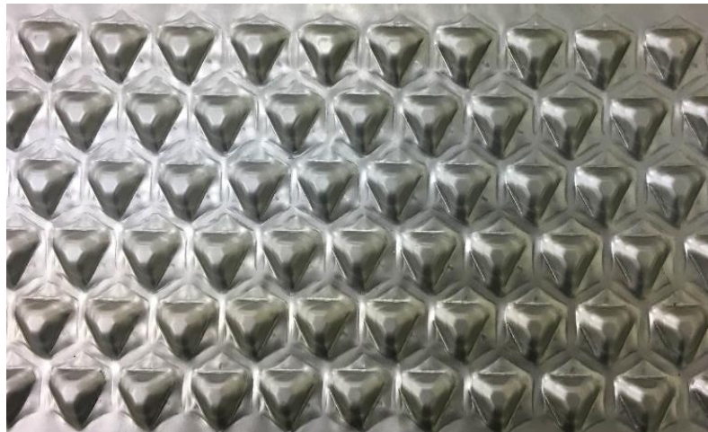
Figure 6.19 Manufactured truss core panel
