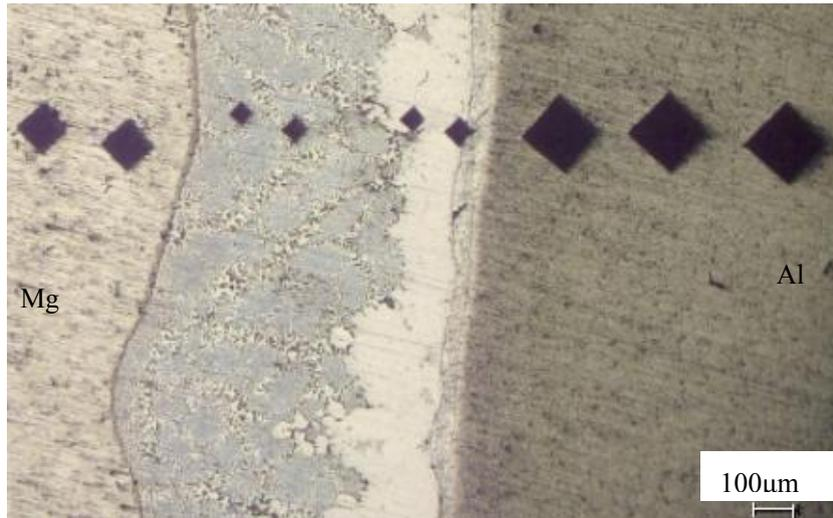
Fig.2.31 The micro-hardness of workpiece annealed at 300°C
