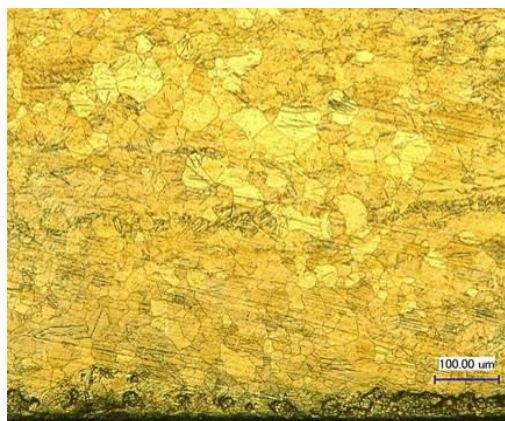
Fig. 4.4 Microstructure of the as-cast strip produced by normal TRC.
