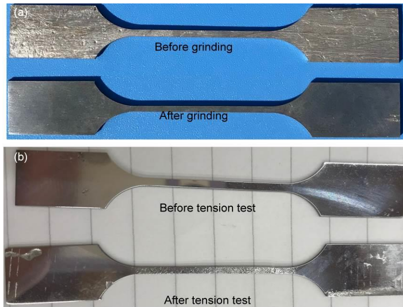
Fig. 4.42 Specimens used for tension test
