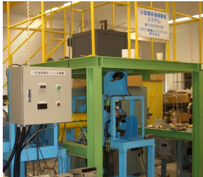
Fig. 3.1 Pilot vertical twin roll caster
