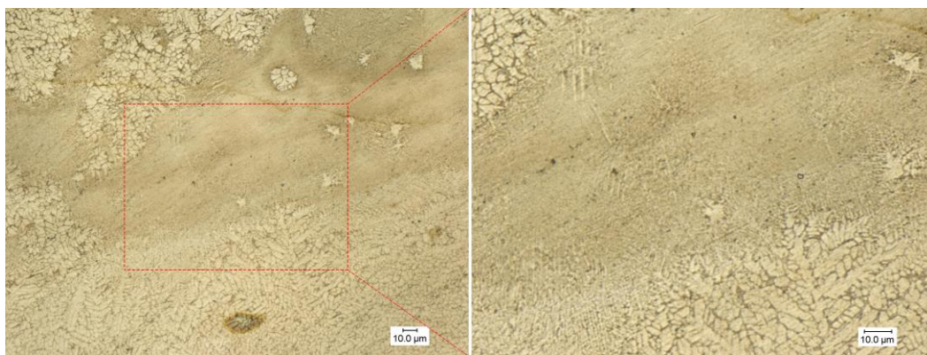
Fig. 4.13 Optical microstructure of the Mg-RE alloy sheet—large quasi-amorphous phase.
