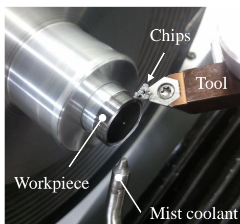
Fig. 3.7 Chip state stagnating during processing of turning.
