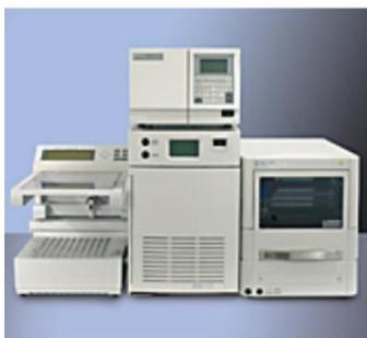
**Figure 1.5** The HPLC system
