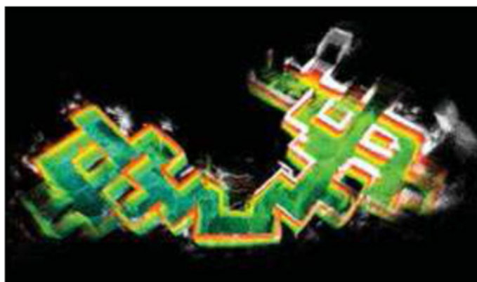
Figure 2-14. A 3D map developed by laser ranger measurements using GraphSLAM. Image courtesy of Keiji Nagatani et al [79]
