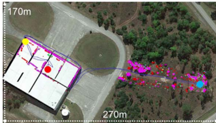
Figure 2-16. The global map and round-trip trajectory overlaid on the Google satellite map in an fully autonomous flight experiment. The blue, red, and yellow dots represents the starting point, goal location, and the only entrance of the warehouse respectively. The global laser point cloud is registered using the estimation produced by the S-MSCKF. Over 700 m trajectory, the final drift is around 3 m under 0.5% of the total traveled distance [87]
