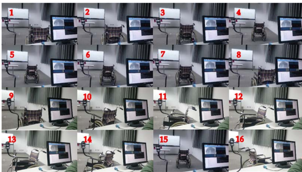
Figure 3-21. Eye blink control wheelchair travel experiment.
