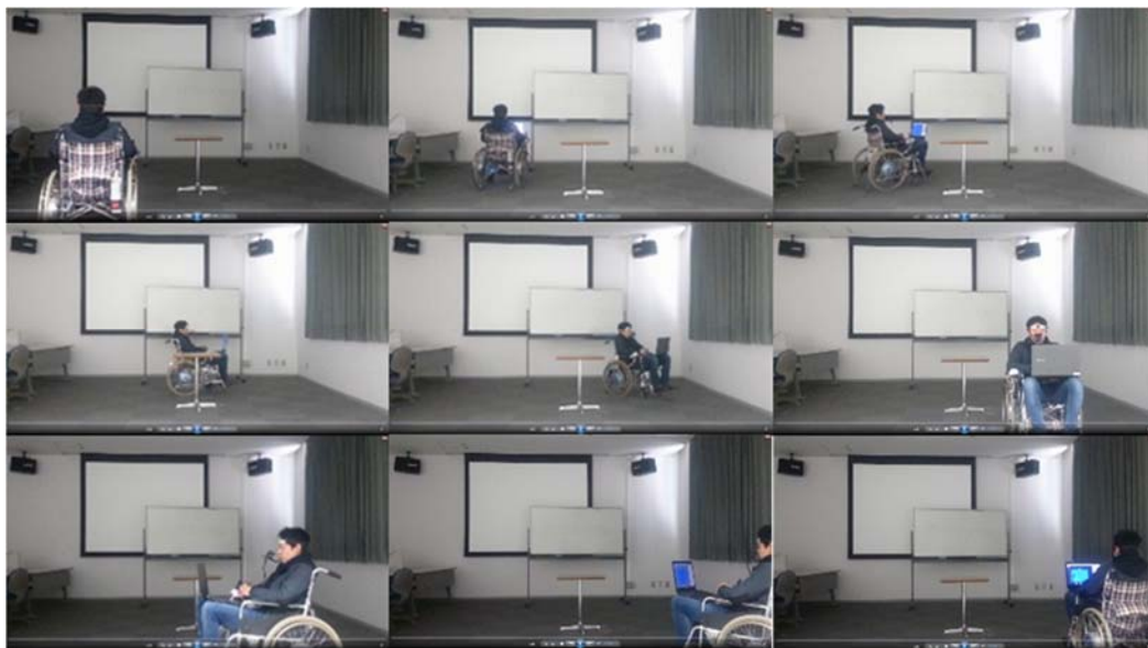
Figure 3-20. Eye gaze direction control wheelchair movement experiment.
