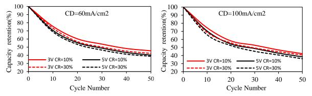
Fig.4.10. The effect of compression ratio and flow rate on discharge capacity retention
