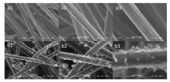
Fig. 3.7 Comparison of SEM images of untreated carbon felts (top) and treated carbon felts
