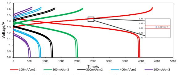
Fig. 4.13 Charge and discharge voltage difference comparison
