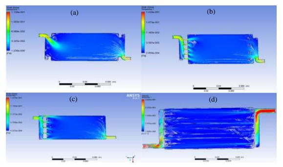
Fig. 4.2. Simulation results of electrolyte flow in the bipolar plate;(a) No flow path;(b)
