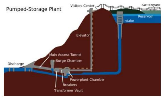
Fig. 1.3 Diagram of the TVA pumped storage facility at Raccoon Mountain Pumped-Storage Plant in Tennessee, United States [18]
