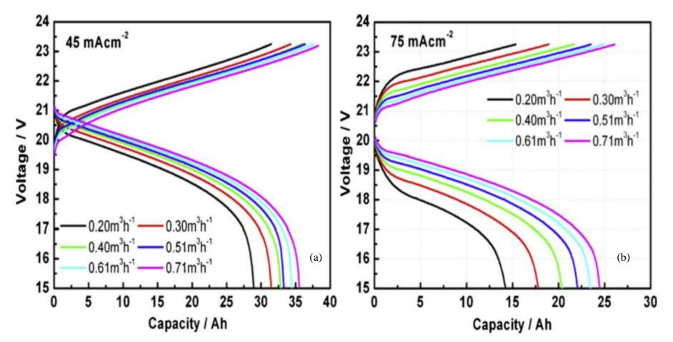
Fig. 2.13. The charge-discharge curves of the battery pack under different electrolyte flow rates. (a) at a charge-discharge current density of  $45 \text{ mA cm}^{-2}$ , (b) at a charge-discharge current density of  $75 \text{ mA cm}^{-2}$ [49].
