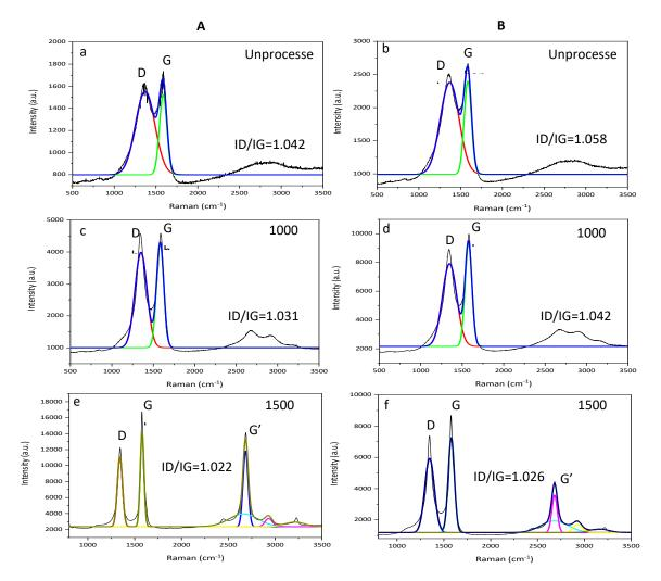
Fig. 3.3. Unprocesse 1000°C and 1500°C heat treatment Raman spectra of two materials Fig. 3.3 e and f Fig. 3.3 f show the Raman after heat treatment at 1500°C. From the figure, it can be seen that with the increase of heat treatment temperature, the D and G peaks have been completely separated, the height of the D peak gradually decreases and the half-value amplitude
