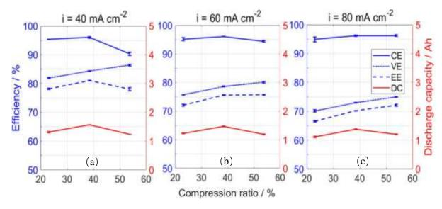
Fig. 2.16.Effect of CR on the coulombic, voltage and energy efficiency and discharge capacity of the VRFB operating at 100 mL min<sup>-1</sup> under various current density levels: (a) 40 mA cm<sup>-2</sup>;
