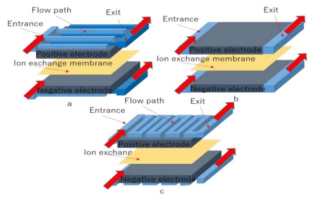
Fig. 2.10 Three different electrolyte flow paths
