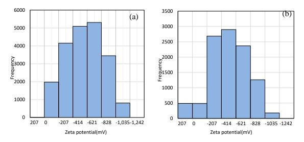
Fig. 3.6 The ZETA potential;(a) 80% ethanol solution,(b)0.1 mol/L (SDBS + 80% ethanol)
