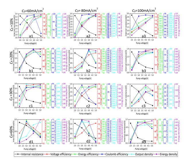
**Fig.4.8**. Comparison of battery charge and discharge performance at different flow rates at the same compression ratio
