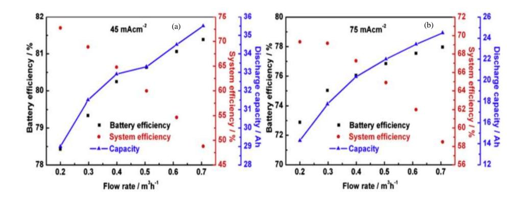
**Fig. 2.14.**The charging and discharging efficiency of the battery pack, the battery power, and the charging and discharging efficiency of the power storage system under different electrolyte flow rates. (a) at a charge-discharge current density of 45 mA cm<sup>-2</sup>, (b) at a charge-discharge current density of 75 mA cm<sup>-2</sup>[49]
