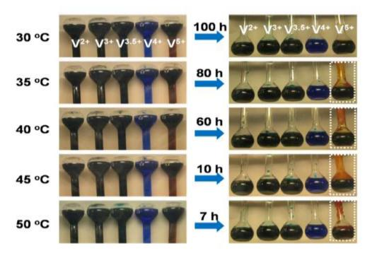
Fig. 2.17. Photographs of five types of electrolytes at high temperature[57].
