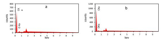
Fig. 3.8 EDS surface elemental analysis results (a: untreated carbon felt b: carbon felt after attachment treatment)
