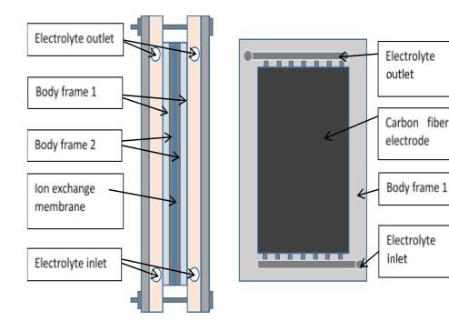
Fig. 4.5. Self-made VRFB framework for experiment
