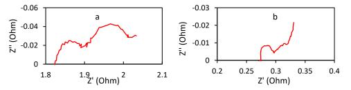
Fig. 3.10 Single battery cell Nyquist figure
