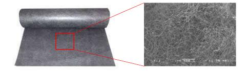
Fig. 2.2 Commercially available carbon felt electrodes
