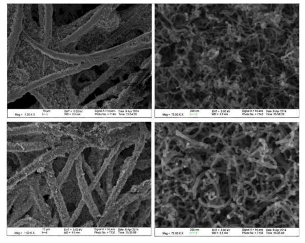
**Fig. 2.3** Pre-soaked carbon electrodes (in CoSO4 and H3BO3) after MWCNT growth a) sample 4 (resynthesized) and b) sample 5. [27]
