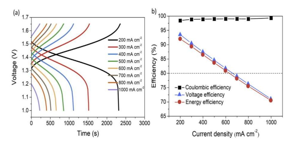
**Fig. 2.4.** (a) The charge-discharge curves of the designed high-performance VRFB at the current densities ranging from 200 to 1000 mAcm<sup>2</sup>. (b) The coulombic, voltage and energy efficiencies of the designed high-performance VRFB[34].
