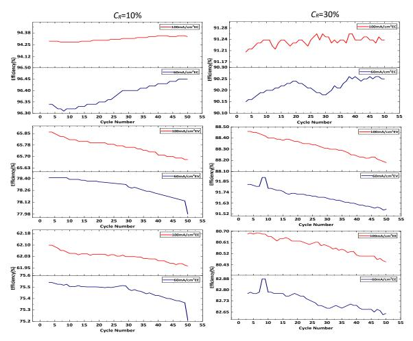
Fig.4.9. Current density of  $60 \text{mA/cm}^2$  and  $100 \text{mA/cm}^2$ , the changes of battery  $E_V$ ,  $E_C$ ,  $E_E$  under different  $C_R$  and  $P_V$  conditions.
