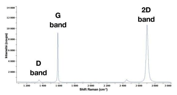
Fig. 3.2. Raman spectra of carbon materials Typical Raman spectra of carbon
