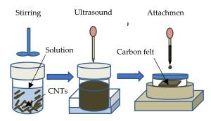
Fig. 3.5 CNTs dispersion and carbon fiber modification
