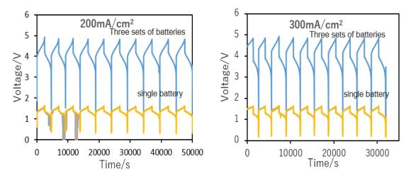
Fig. 4.14 200 mA/cm<sup>2</sup> and 300 mA/cm<sup>2</sup> continuous charge and discharge
