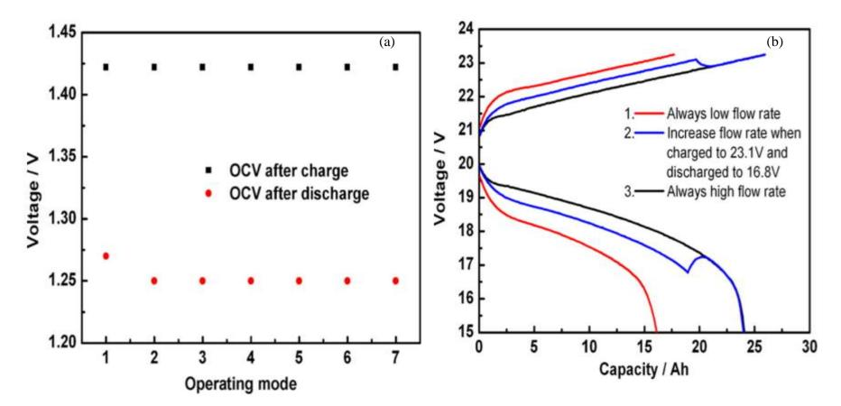
**Fig. 2.15.**(a) OCVs after charge process and discharge process at different operating modes when using an optimal strategy of flow rate for charge process. (b)Charge–discharge curves atdifferent operatingmodes when using an optimal strategy of flow rate for discharge process[49]
