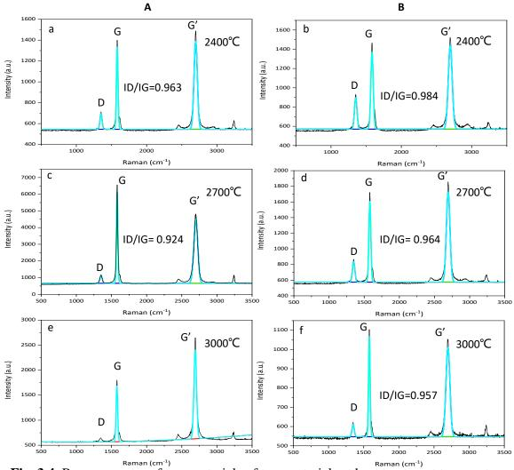
**Fig. 3.4.** Raman spectra of two materials of two materials at heat treatment temperatures of 2400°C ,2700°C and 3000°C
