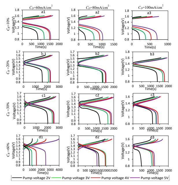
**Fig.4.7**. Charge and discharge data with different current densities, different compression ratios, and different electrolyte flow rates.
