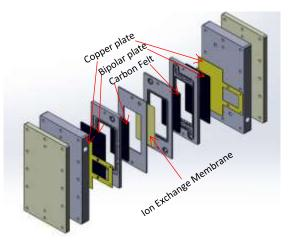
Fig. 4.1. Internal structure of the battery
