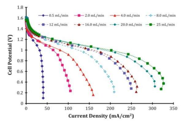
Fig. 2.12. Polarization curves of batteries at different electrolyte flow rates [48].
