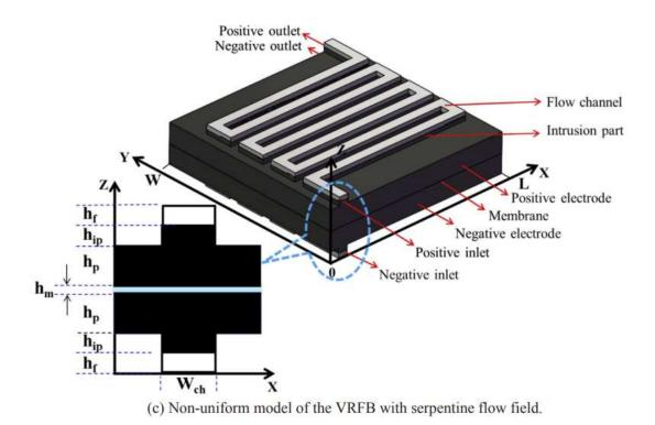
Fig. 2.11. Geometric model for the non-uniformly compressed electrode. [45]
