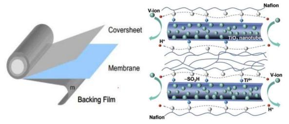
Fig. 2.7 Ion exchange membranes and how they work
