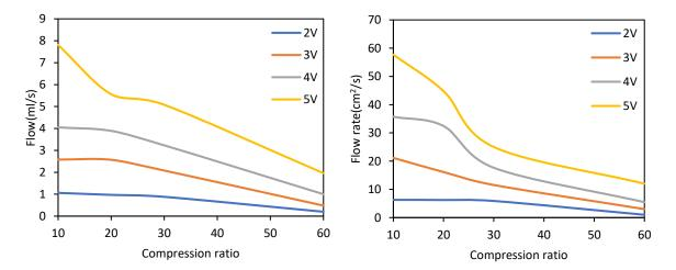
**Fig.4.6** The relationship between pump input voltage and flow rate with different compression ratios of 4mm carbon fiber.
