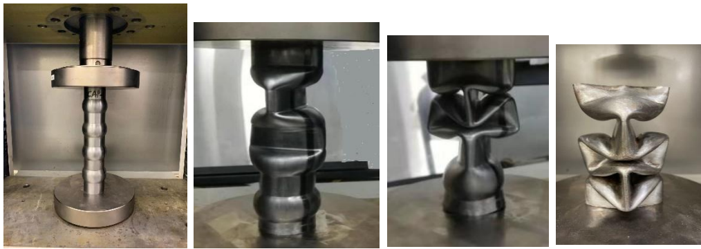
Figure 4.30 Experimental configuration and various crushed states of the CAP during its deformation.
