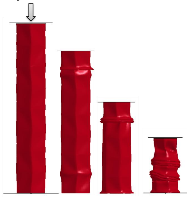
Figure 3.16 Results of crushing deformation at a rotation of 5°
