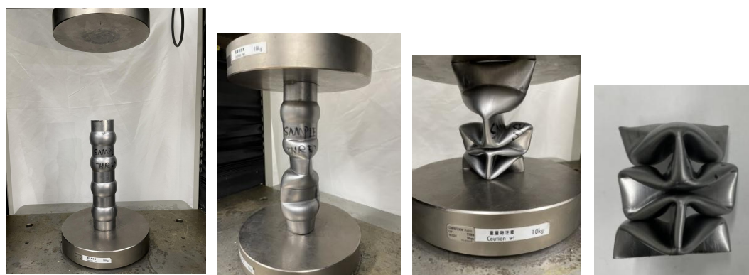
Figure 5.29 Experimental configuration and various crushed states of the CAP during its deformation
