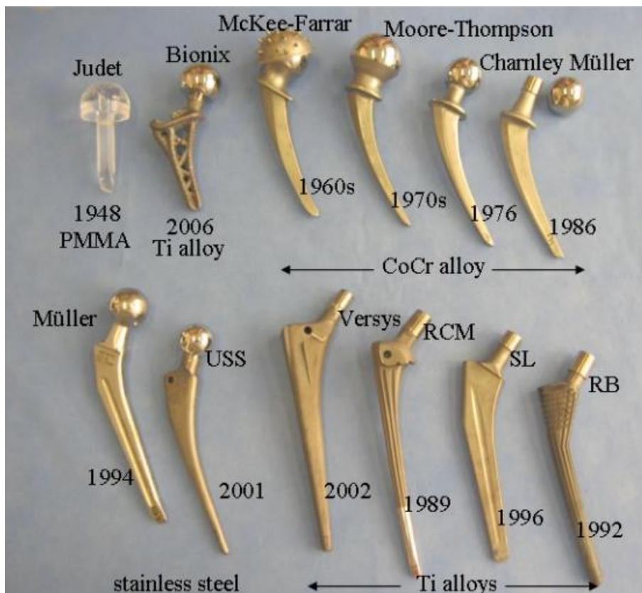
**Fig. 1.1** Examples of older and recent types of hip prostheses made of PMMA, stainless steel, Co- and Ti-based alloys. For each prosthesis, the year of manufacture is denoted [2].
