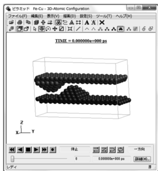
Fig. 3 Simulation image of the elementary process of friction and wear with MD method (Materials Explorer 5.0).
